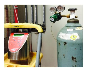
Utilization: Introduce the sparging stone through the top of the tank or an insertion tube from the bottom valve. The machine doses continuously introducing O2 precisely (by weight, not by volume).
