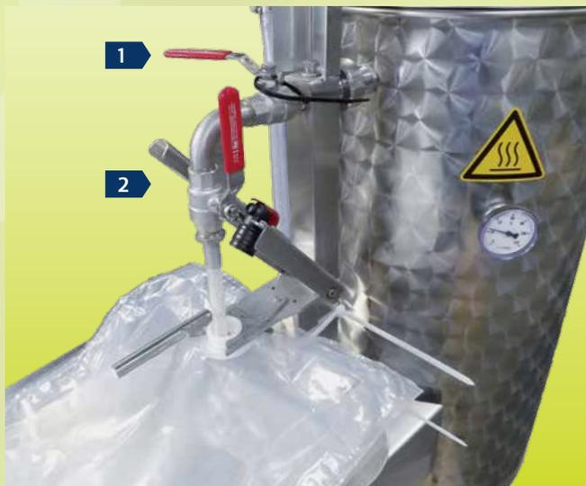
**1 Bottle filling:** The pasteurisation temperature is controlled by using a ball valve to regulate the flow rate. The filling is started and stopped by self-actuating valves when the bottles are placed and removed.
