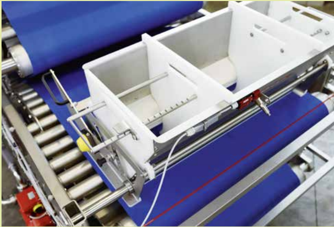
Adjustable (width, height) mash application roller results in a symmetrical mash-film.
