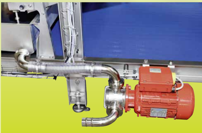
The swift pressing process, low fall height and rapid draining of the strained juice into the small volume main juice collection trough reduces oxidation to a minimum.
